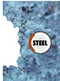
Remove spalled concrete from deteriorating structure.
